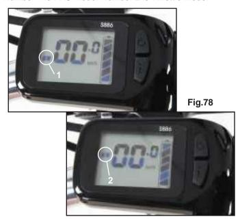
c) Press the power button and function button at same time, you can switch the speed unit between km/h and mph.
