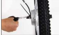
2) Remove two screws at front dropout (Fig.15).
