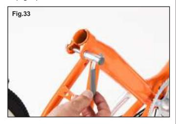
Insert the seat into frame. Adjust the seat height up or down until the rider feels they have control of the tricycle and are comfortable. Ensure the seat is securely locked in place (Fig.34).
