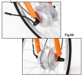
3) Connect the cable of motor, align the arrow at cable head (Fig.69).
