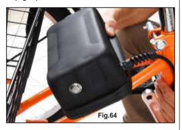
2) Tighten the battery box by screws or cable tie (Fig.65).
