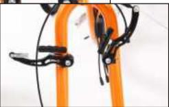
4) Place the front tire into the fork openings. The motor cable is at right side (Fig.17). Be sure both sides of the axle rest on the fork and the tire is centered (Fig.18).
