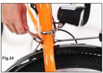
Note: if any bending of front fender, bend it to opposite direction a little and then make it at center.
