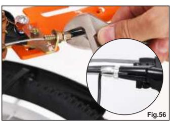
10) If still not brake the tire, try to loosen the nut which fixed cable head a little. And pull the brake lever further, and then close the nut. Repeat the step 9) again.
