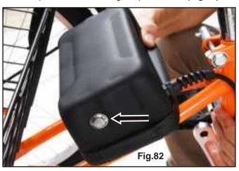
2) Open the zipper, open the cover of battery box. You could insert the battery in the mounting plate (Fig.83).
