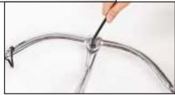
2) Loosed the clamping screw in the middle with 6mm Allen wrench. Turn up the handle bar to a comport holding angle, and then close the screw (Fig.9).
