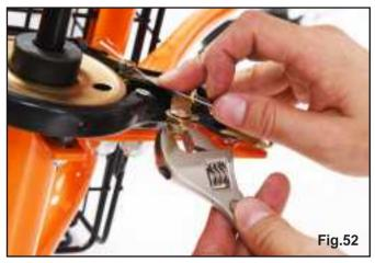
7) Insert cable head through the hole of at the bolt **(Fig.53)**.
