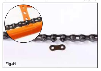
4) Clamp the clipping washer at the outside of plate. Ensure the post pin be locked firmly (Fig.42).
