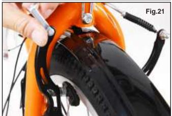
2) Assemble the brace arm of front fender to the front dropout at both sides. Loosely tighten the screws (Fig.22).
