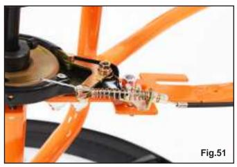
6) Loosen the fixing nut, if necessary, you can remove the nut **(Fig.52)**.
